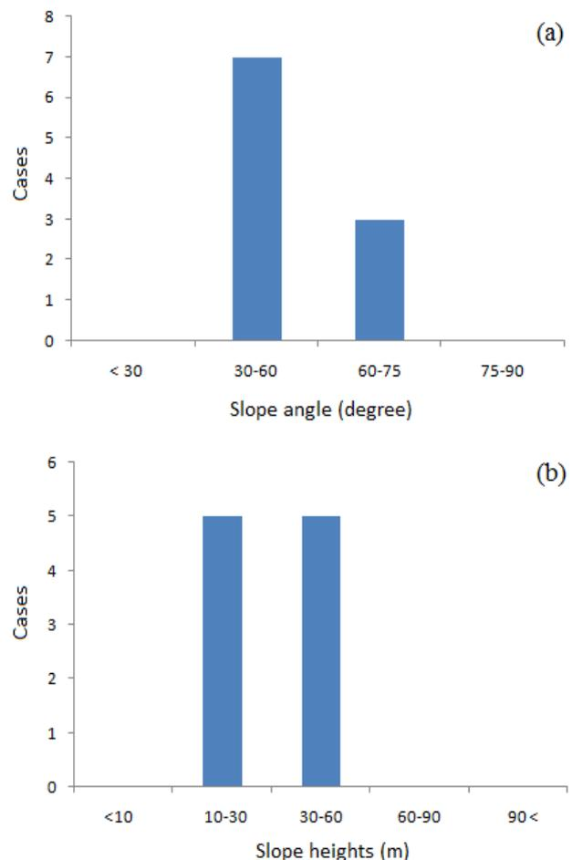
**Figure 5.** Data-set of the studied slopes for the Q-slope parameters: (a) slope angle variation, (b) slope height variation
