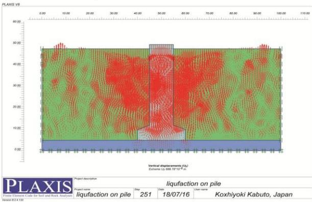
Figure 4. The displacement state during the liquefaction event
