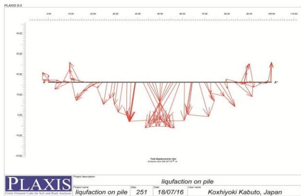
Figure 12. The displacement vectors state as the soil liquefies perpendicular to the pile
