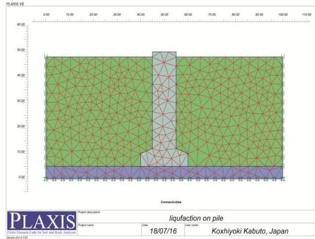
Figure 3. Model prepared after assigning materials properties
