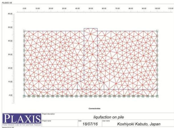
Figure 2. Model prepared from the embankment boundary conditions under study (free and viscous boundaries)
