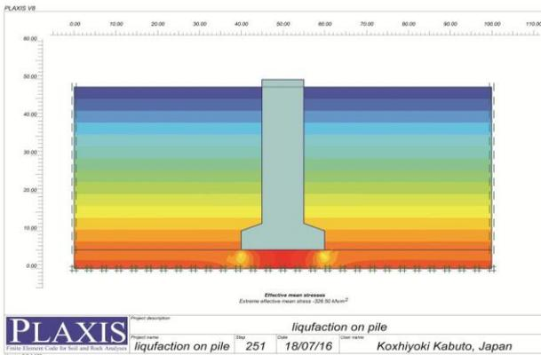
Figure 11. The shear stress state of liquefaction inhibition on pile
