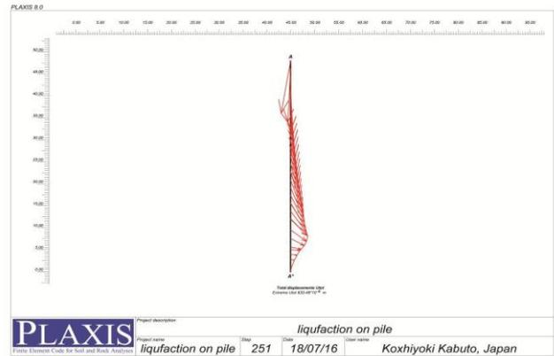
Figure 13. The displacement vectors state as the soil liquefies parallel to the pile
