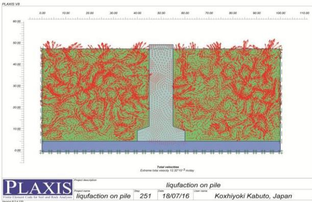
Figure 5. The velocity state during the liquefaction event
