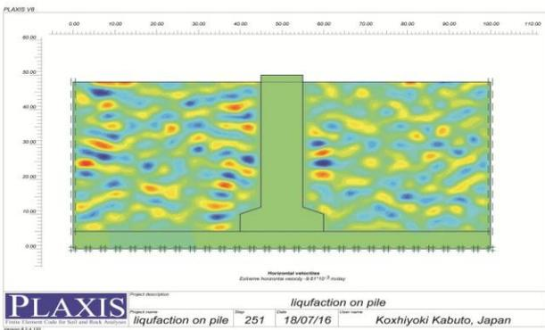
Figure 6. The stress field state during the liquefaction event
