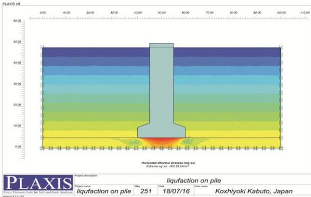
Figure 10. The main stress state of liquefaction inhibition on pile
