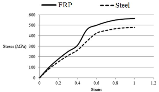
**Figure 10.** Crack stress-strain curve in two types of reinforcement in seismic loading
