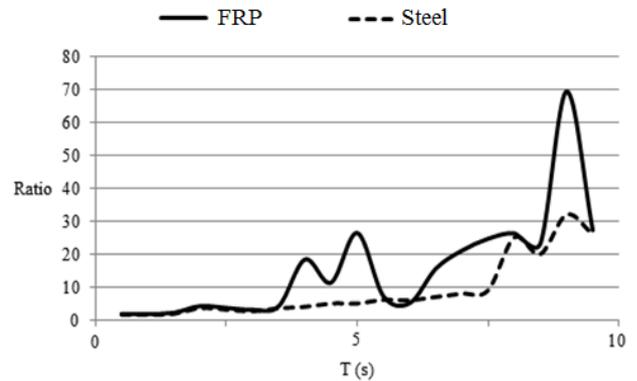
Figure 7. Van-Meiss tension ratio at the crack edge in two types of reinforcement
