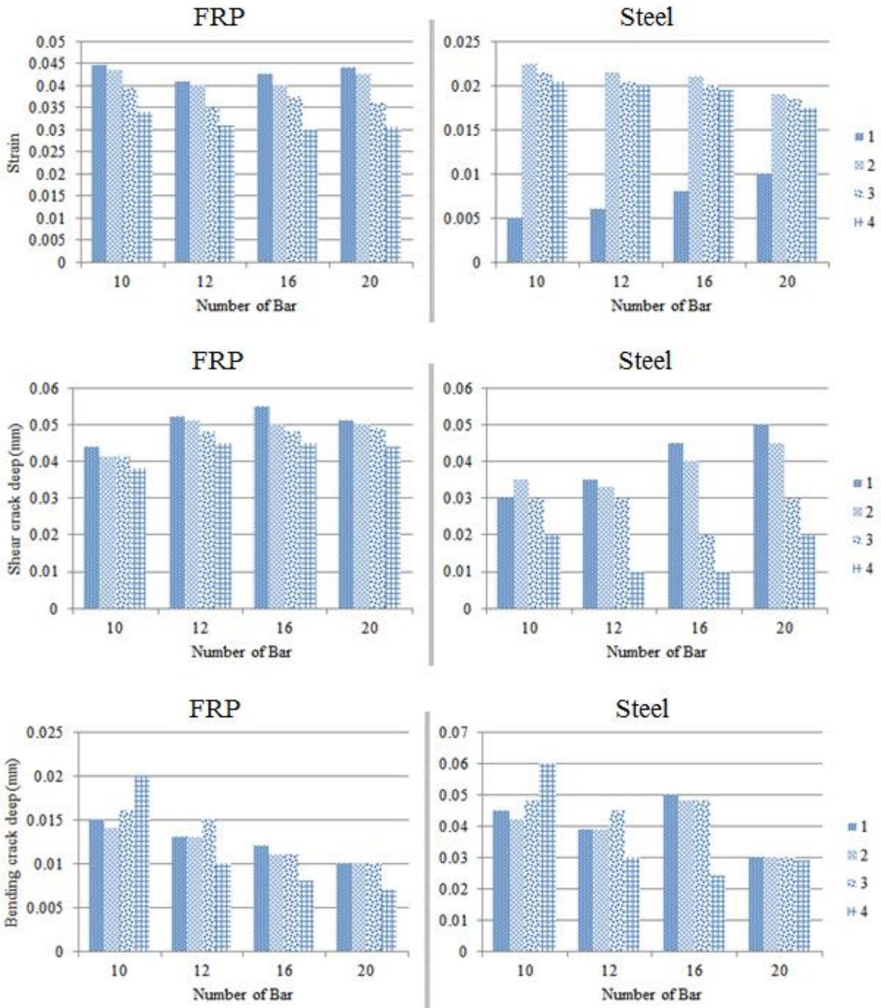
Figure 12. Changes in the number of reinforcements and the shear crack depth of the frame in two samples (FRP/Steel)
