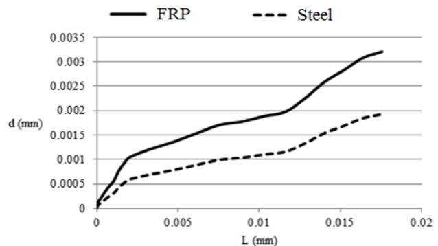
Figure 8. Increasing the diameter of the crack opening in terms of the ratio of crack length in concrete
