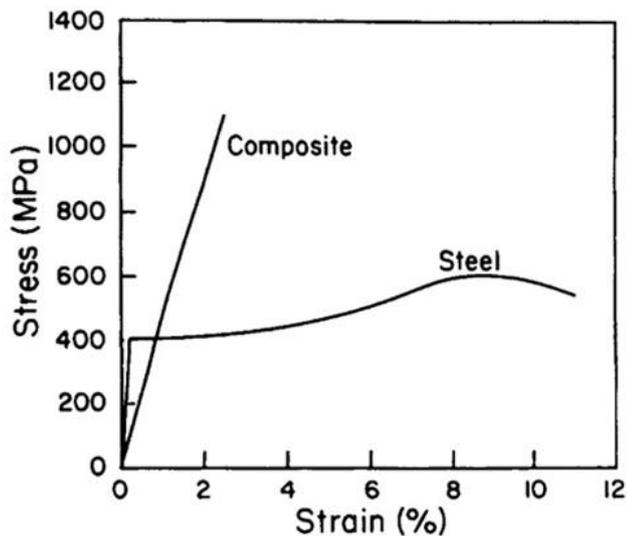
Figure 1. Stress-Strain curve of composite vs. steel reinforcements (Shin et al., 2020)
