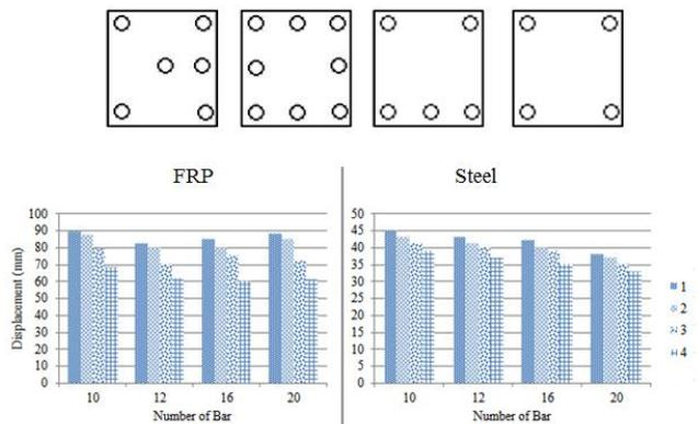
**Figure 11.** Number of reinforcements and frame rise in two examples of FRP vs. steel
