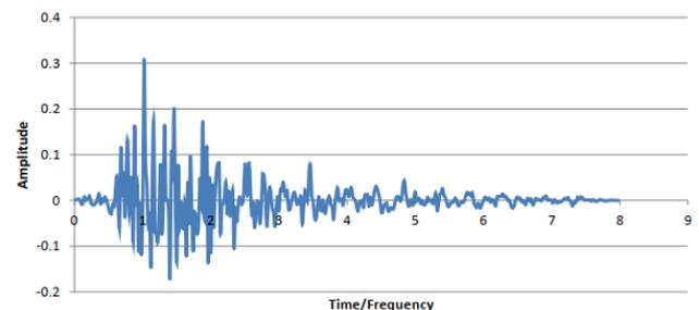
**Figure 3.** Earthquake load profile applied to the structure
