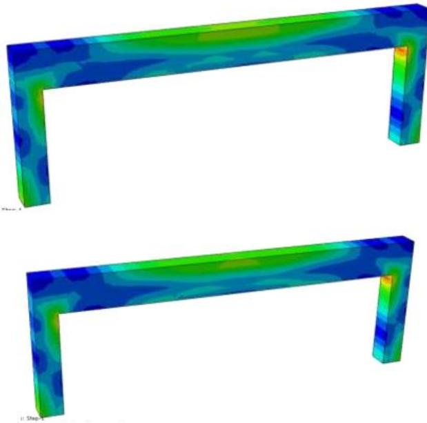
Figure 6. Stress distribution in the concrete frame
