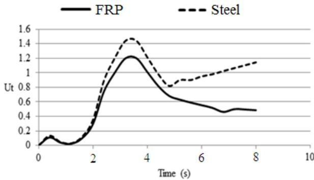
**Figure 9.** Ratio of crack edge displacement to seismic load displacement in concrete
