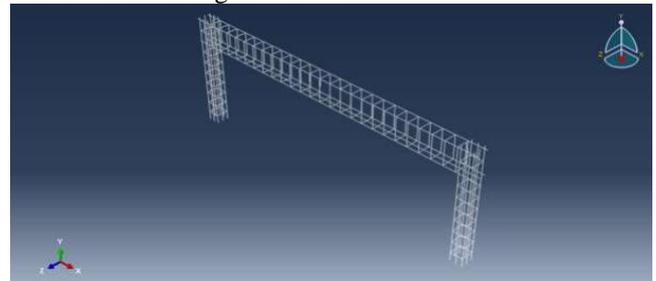
**Figure 2.** The geometry of reinforced concrete with FRP
