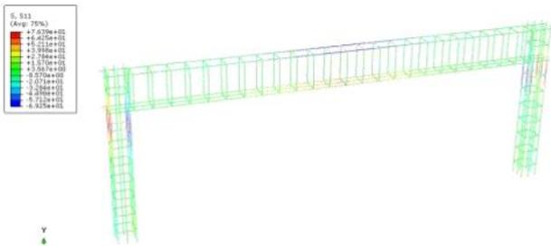
Figure 5. Stress distribution in composite reinforcements
