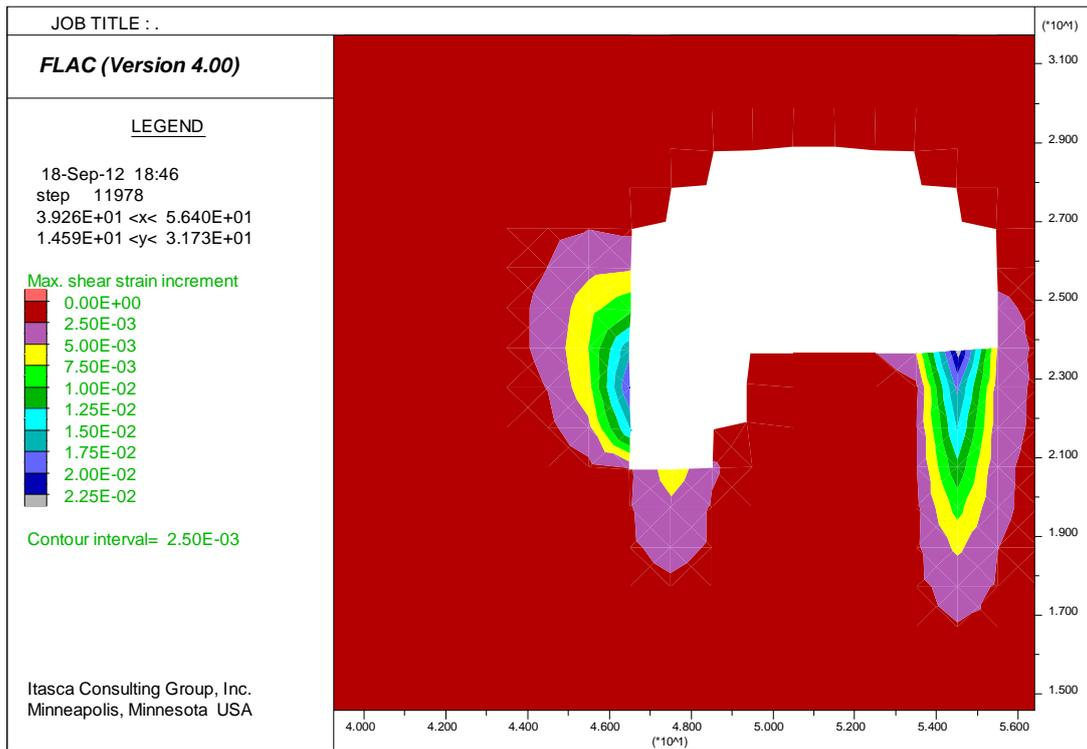
Fig. 14 Shear force developed after excavation of the left cut wall
