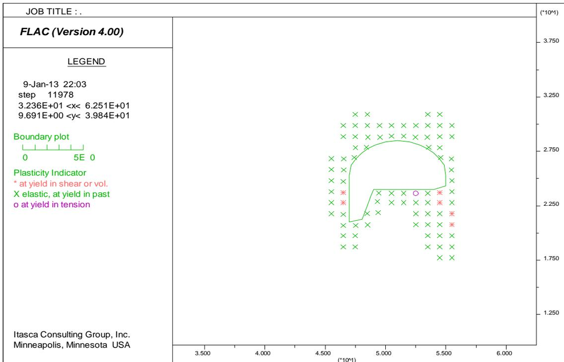
Fig. 15 Expansion of the plastic zone after excavation of the left cut wall
