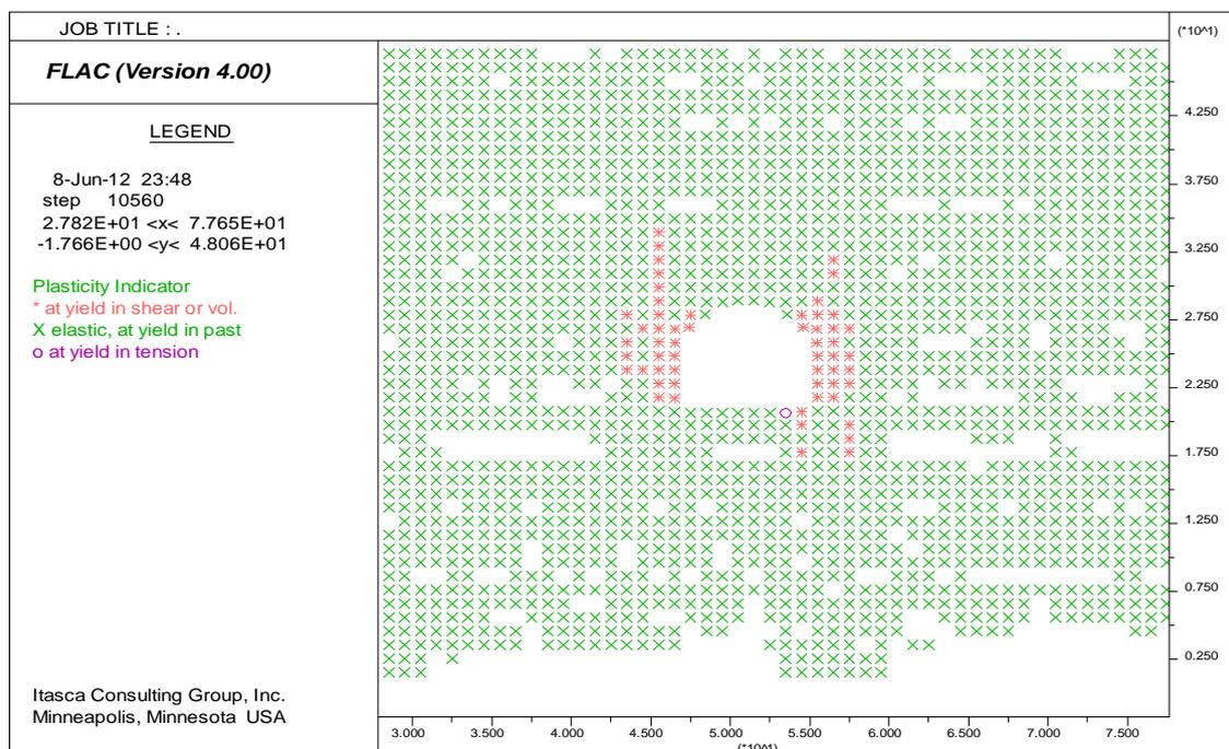
Fig. 7 Expansion of the plastic zone around the section
