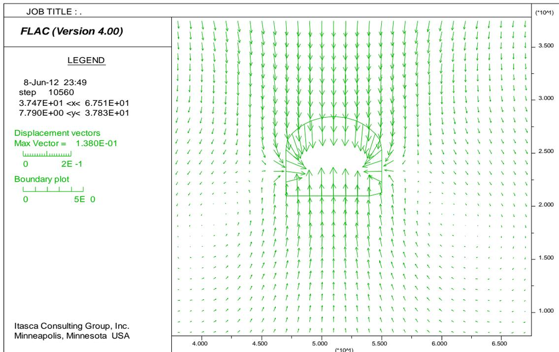
Fig. 6 The tunnel displacement contour; single stage
