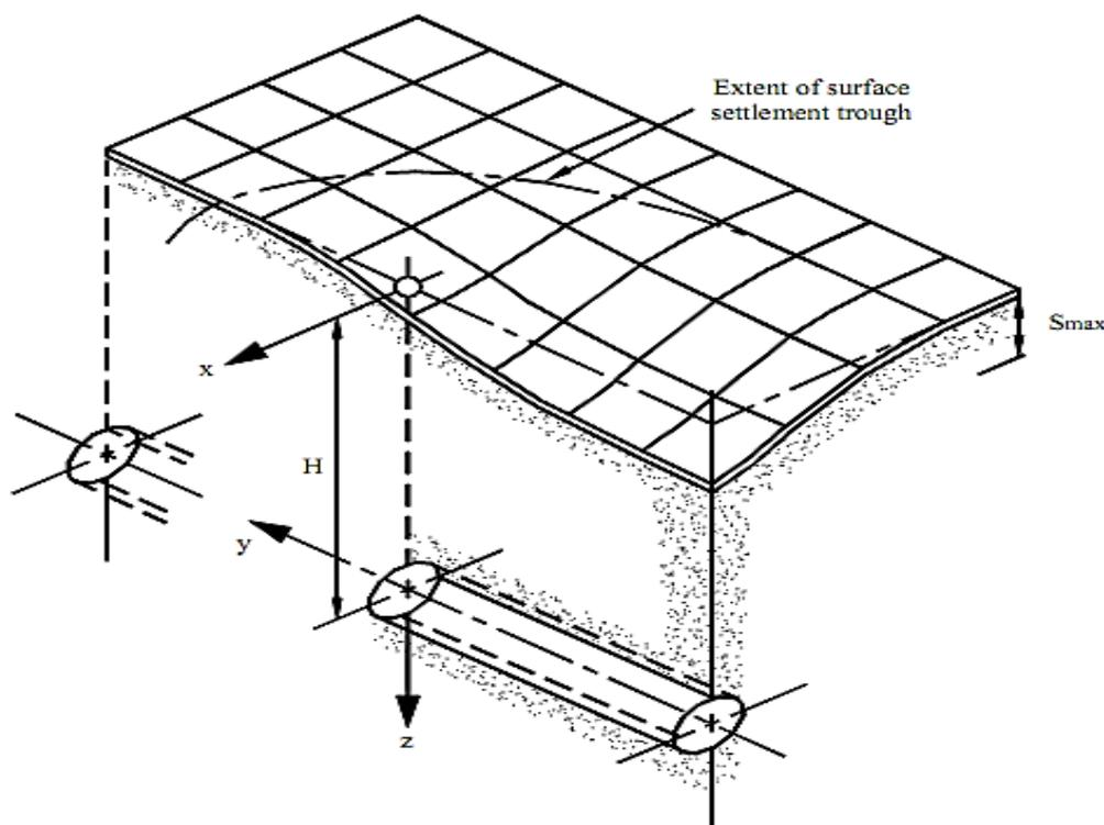
Fig. 1 Three-dimensional distribution of the settlement due to the tunnel excavation (Leca et al. 2002)
