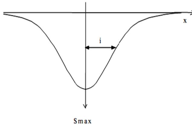
Fig. 2 Surface settlement profile (Leca et al. 2002)
