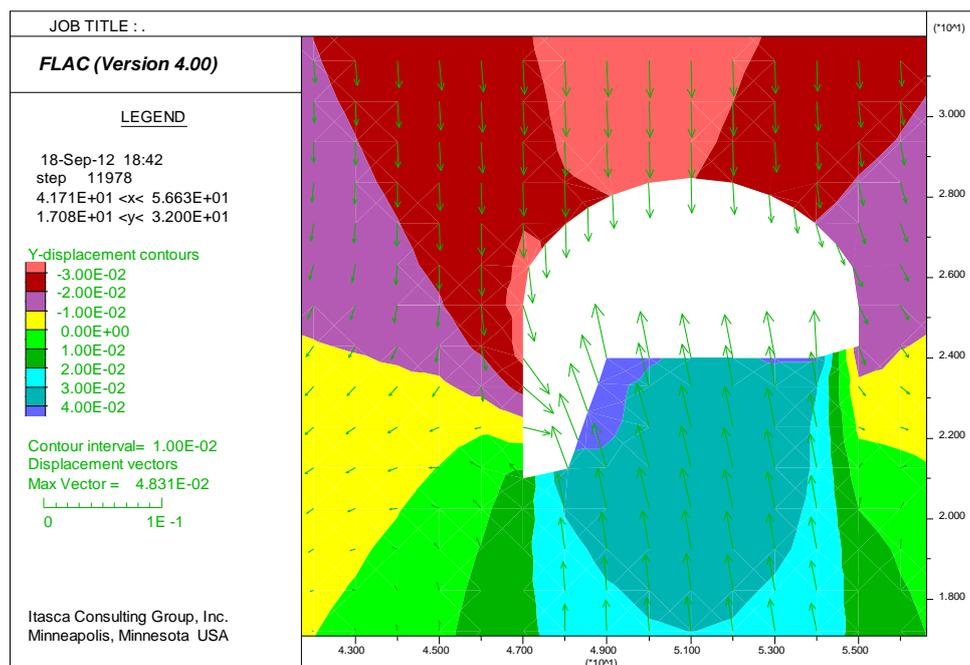
Fig. 13 Vertical displacement after excavation of the left cut wall
