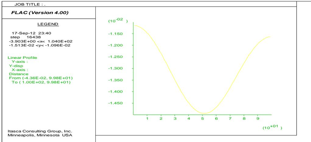
Fig. 10 Settlement in the section
