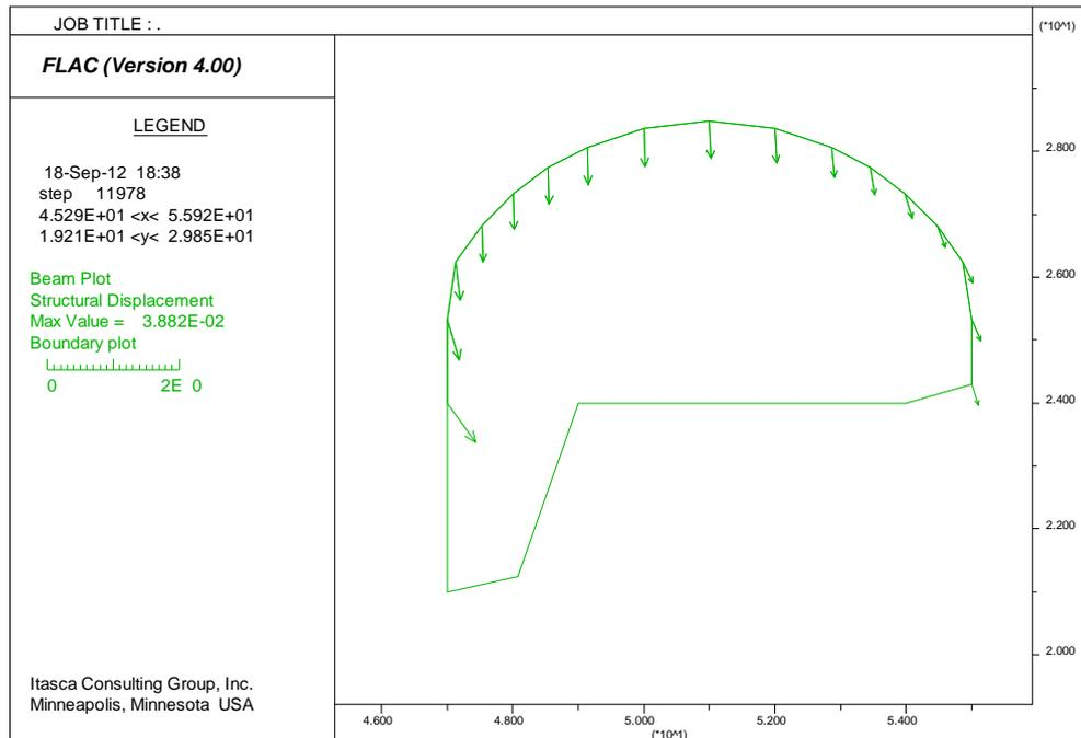
Fig. 12 Shot Crete displacement after excavation of the left cut bank
