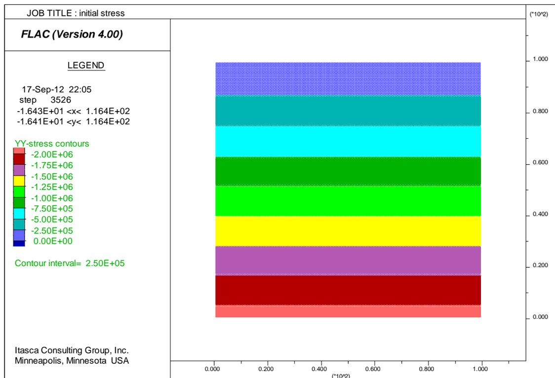
Fig. 5 The in-situ stress before tunnel drilling
