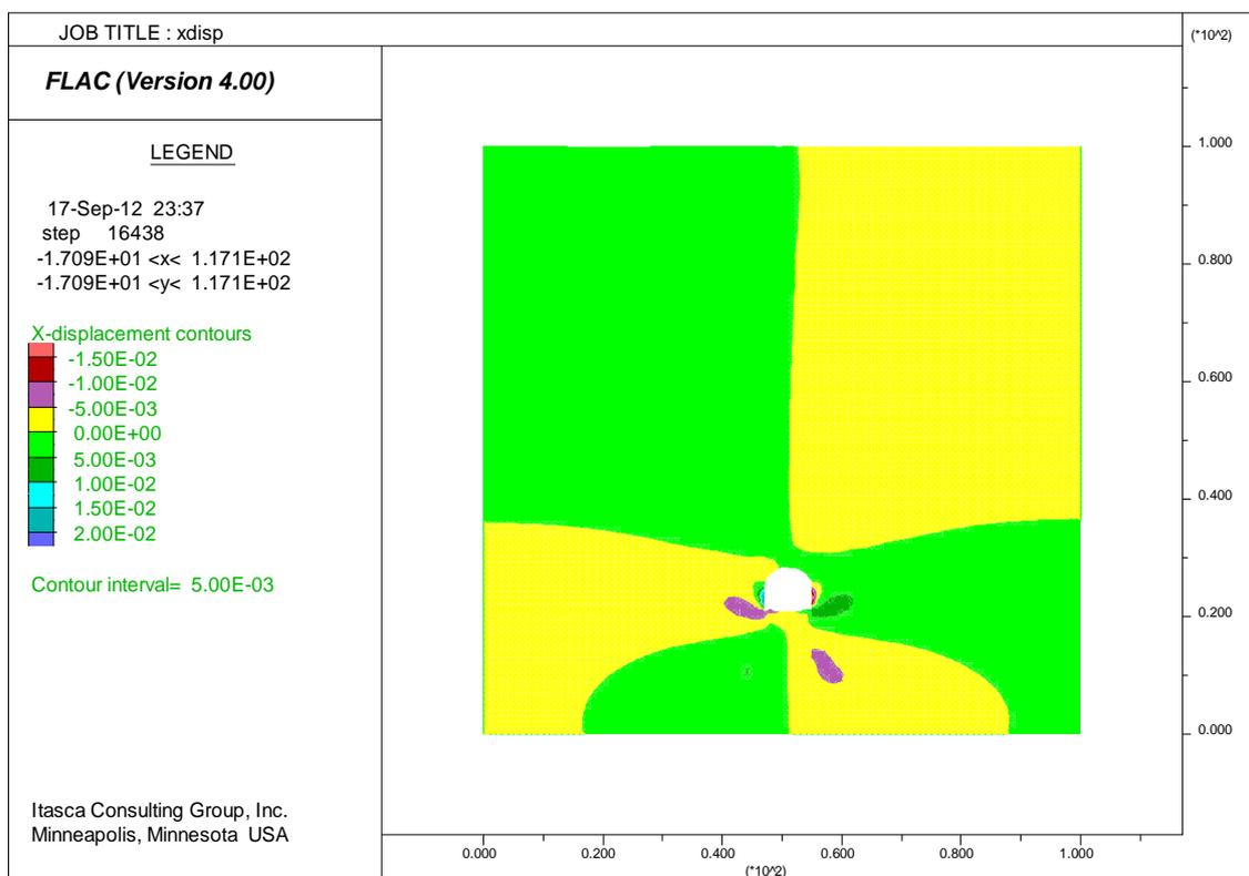
**Fig. 9 The horizontal displacement around the tunnel section**
