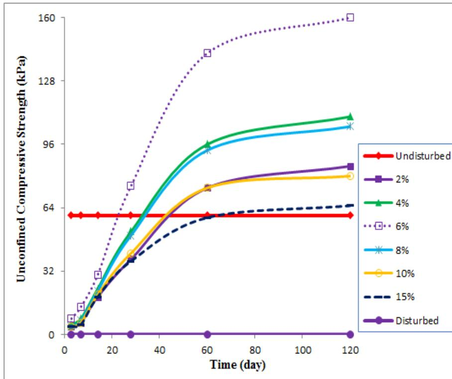
Figure 6 Changes of compressive strength of the soil sample with different ratios of lime to the time
