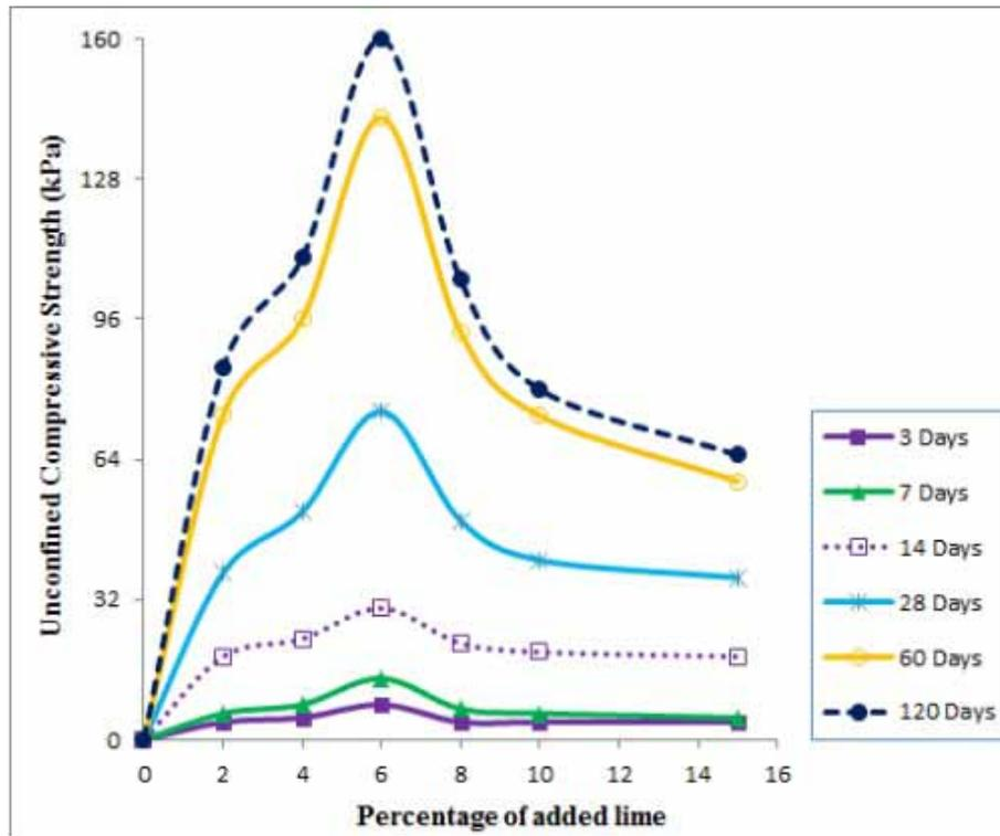
Fig. 8 Changes of compressive strength of the soil sample in different times to the lime ratio
