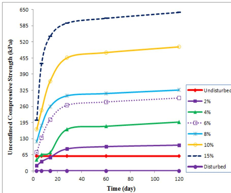
Figure 5 Changes of compressive strength of the soil sample with different ratios of cement to the time
