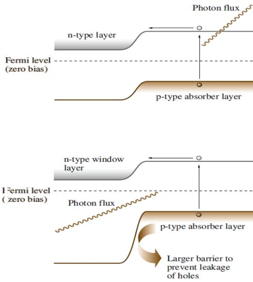
Figure 2. Schematic of an energy-band diagram for a standard solar cell (Kasap and Capper, 2017)
