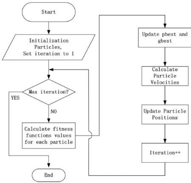
Figure 5. PSO and P&O application flowchart (Qin and Kimball, 2011)
