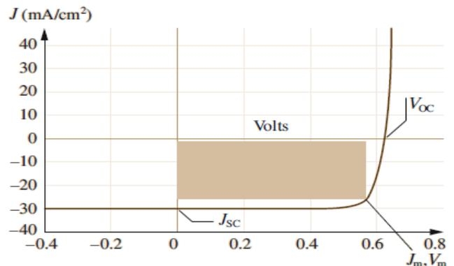
Figure 3. Ideal J–V characteristic for a PV cell
