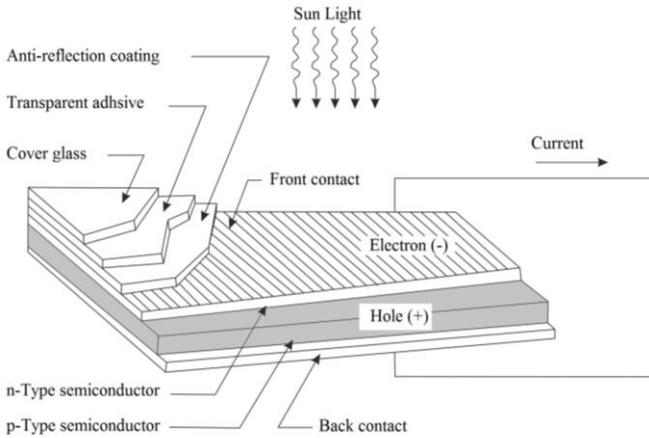
Figure 1. The mechanism of the PV system (Xiao, 2017)
