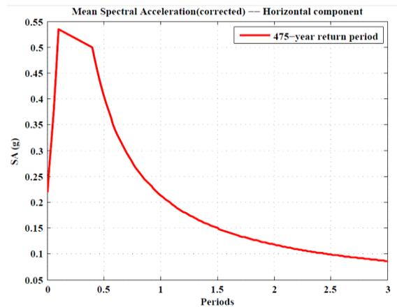
Figure 6. The corrected horizontal acceleration spectrum in different periods for 475 returns period
