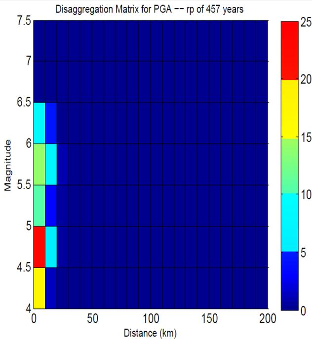
Figure 4. Analytical separation for 475 as return period (in maximum acceleration). The dominant scenario in distance and magnitude point of view is indicating by colorful cells
