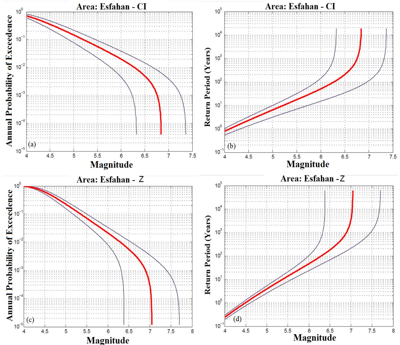
**Figure 2.** Possibility for the occurrence of an earthquake with different magnitude using Gardner Knopoff (1974) method (for CI and Zagros in Panel 1 and 3, respectively), The average annual return period for earthquake in different magnitude using Kijko-Sellevoll method (for CI and Zagros in Panel 2 and 4, respectively).
