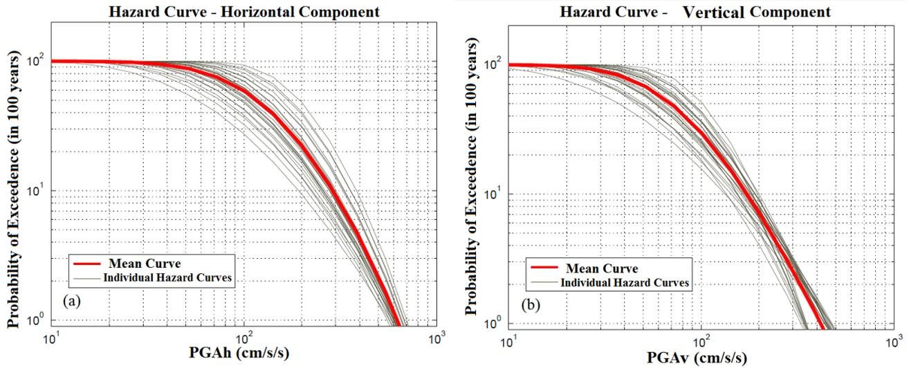
Figure 3. Possibility of experiencing maximum horizontal acceleration (first panel) and vertical acceleration (second panel) in study region
