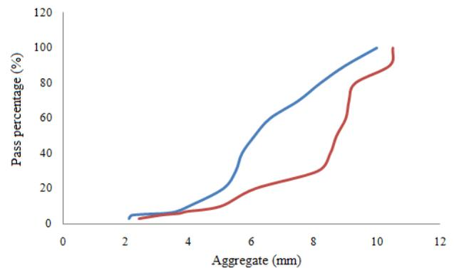
**Figure 1.** Particle-size distribution of aggregate
