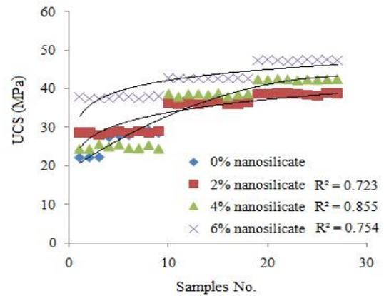
Figure 16. Regression analysis of nanosilicate vs UCS in samples
