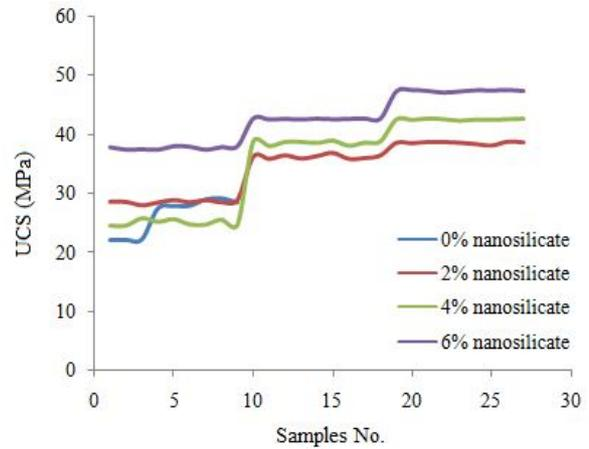
Figure 15. Variation of nanosilicate vs UCS in samples
