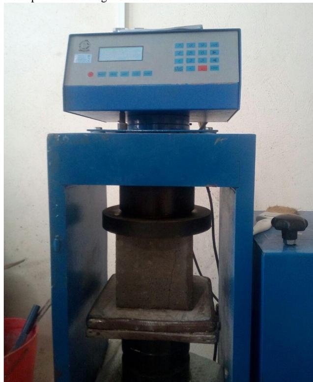
**Figure 3.** The UTM test device
