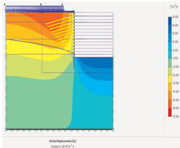
Figure 7. Vertical counterdisplacement of northern wall in nailing method inside Plaxis
