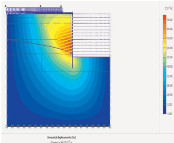
Figure 8. Horizontal counter displacement of northern wall in nailing method inside Plaxis
