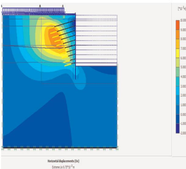
Figure 10. Horizontal counter displacement of northern wall in anchoring method by Plaxis
