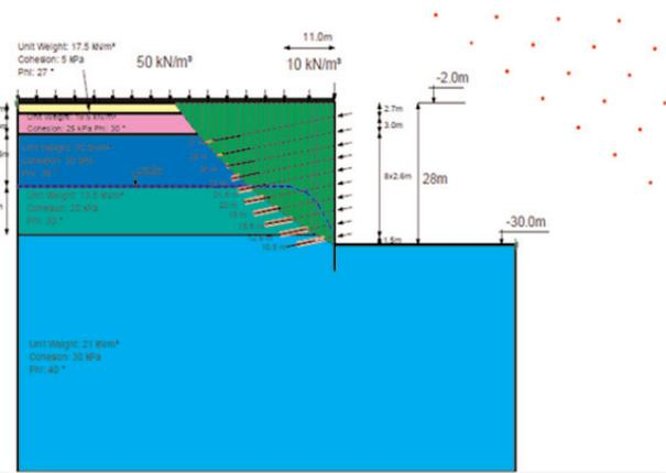
Figure 6. Geoslope output in the northern wall with the safety factor 1.522 by anchorage method
