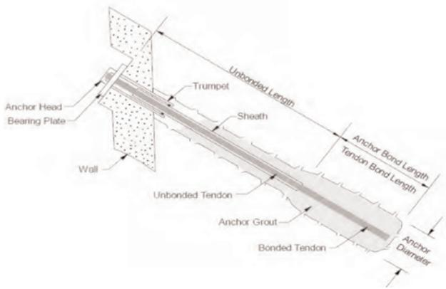
Figure 1. Components of ground anchor
