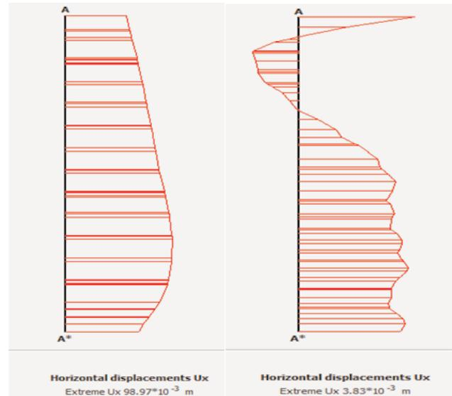
Figure 11. Diagram for the horizontal displacement of wall in nailing system (on the left) and anchoring (on the right)
