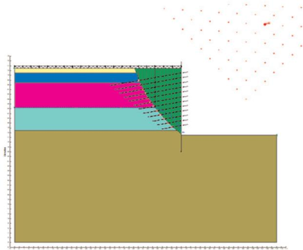
Figure 5. Geoslope output in the northern wall with the safety factor 1.1 by nailing method
