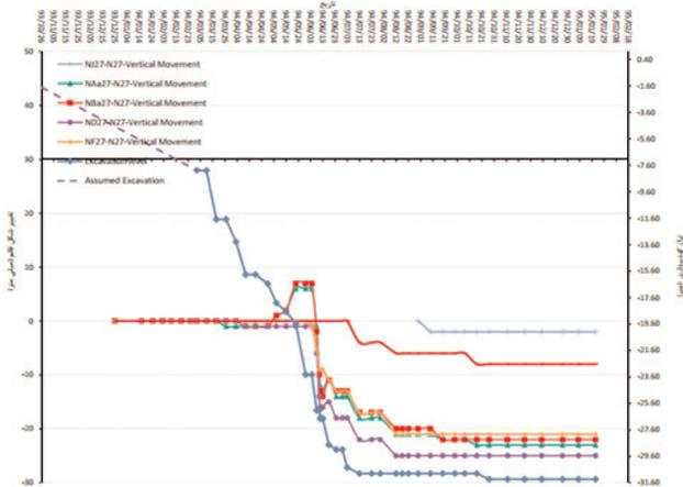
Figure 4. The diagram for the vertical deformations of northern wall using anchoring
