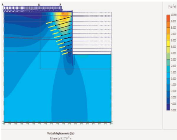
Figure 9. Vertical counter displacement of northern wall in anchoring method by plaxis
