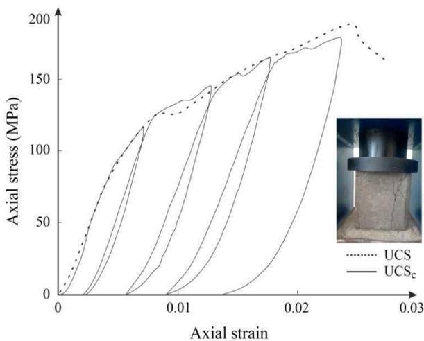
Figure 8. UCS<sub>c</sub> test steps and results (cycle 4)
