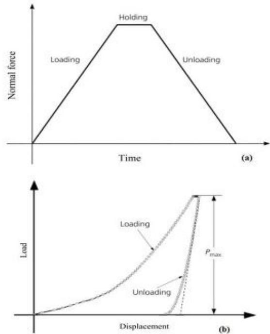
Figure 4.  $UCS_c$  test work process: (a) loading-unloading in a cycle, (b) recorded data/results of cycle
