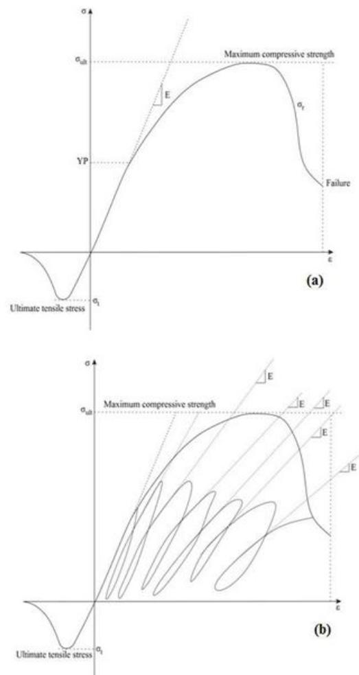
**Figure 1.** The behavior of the elastic materials like concrete: (a) Topical behavior of concrete, (b) Fatigue behavior of concrete
