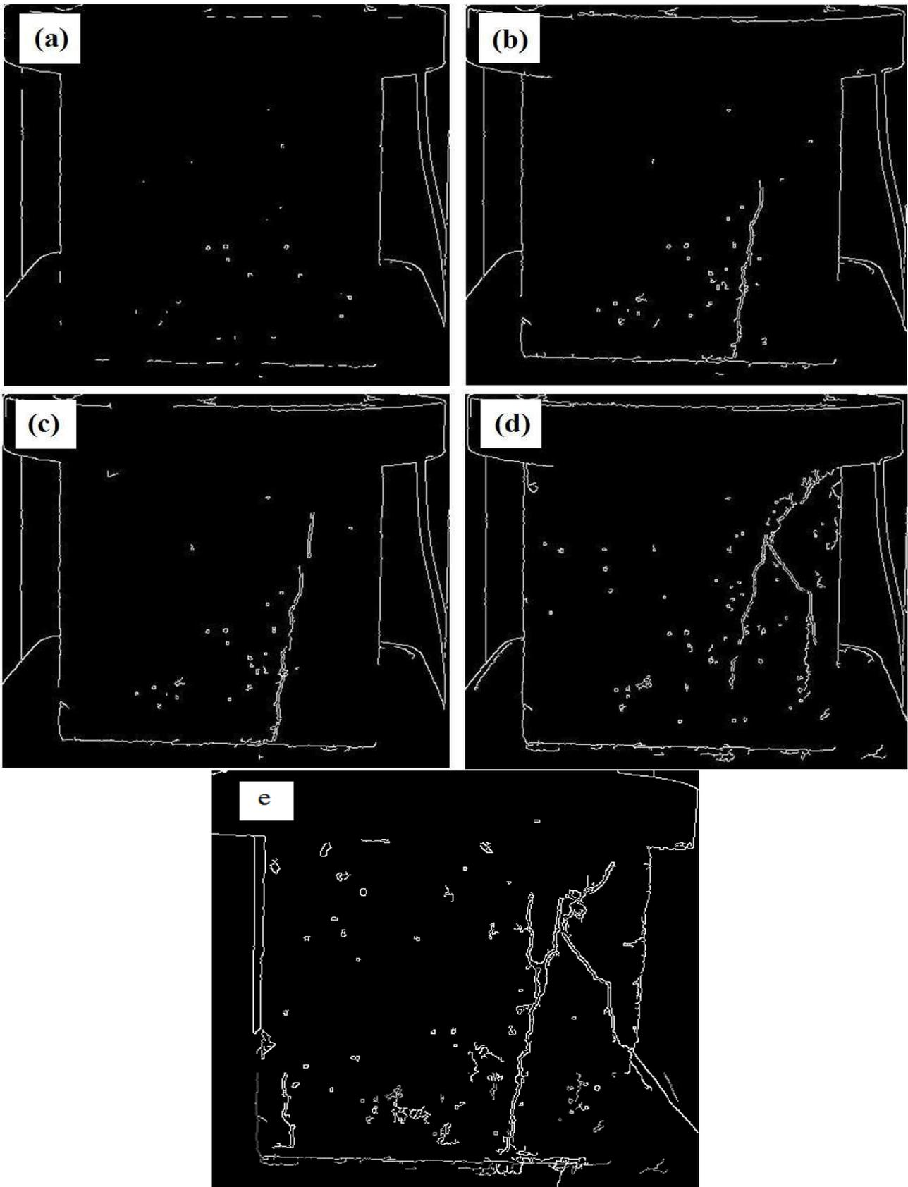
**Figure 10.** Crack propagation by IPT, (a) cycle 1, (b) cycle 2, (c) cycle 3, (d) cycle 4, (e) cycle 5
