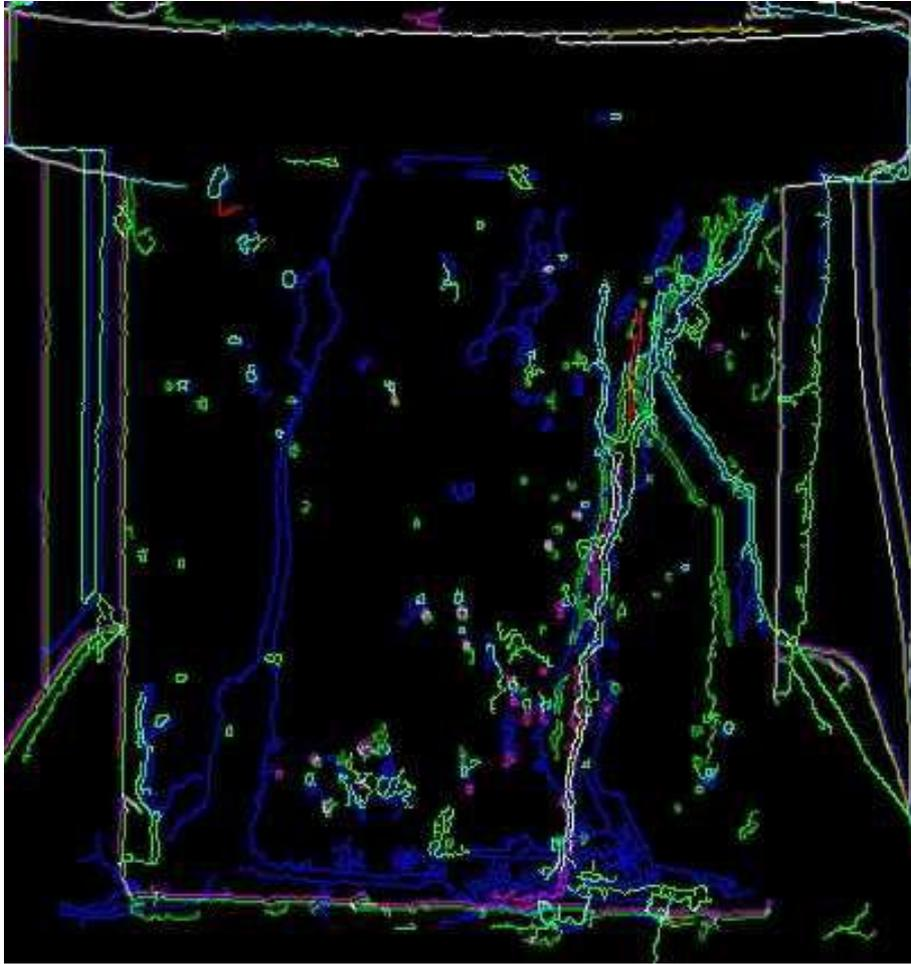
**Figure. 11.** The model of crack propagation in concrete specimens under UCS.
