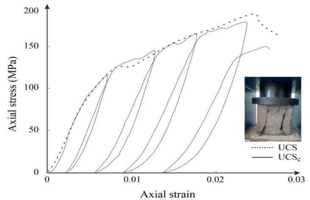
Figure 9. UCS<sub>c</sub> test steps and results (cycle 5)
