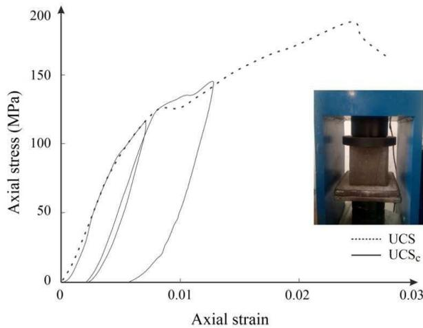
Figure 6. UCS<sub>c</sub> test steps and results (cycle 2)
