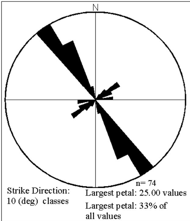
**Fig. 9-** Most parts of the Sistan plain and so with the lineaments are covered by alluvium. Analysis of the not covered lineaments show, mainly fractures with a NW irection, which confirms fracturing through bending of the structure.
