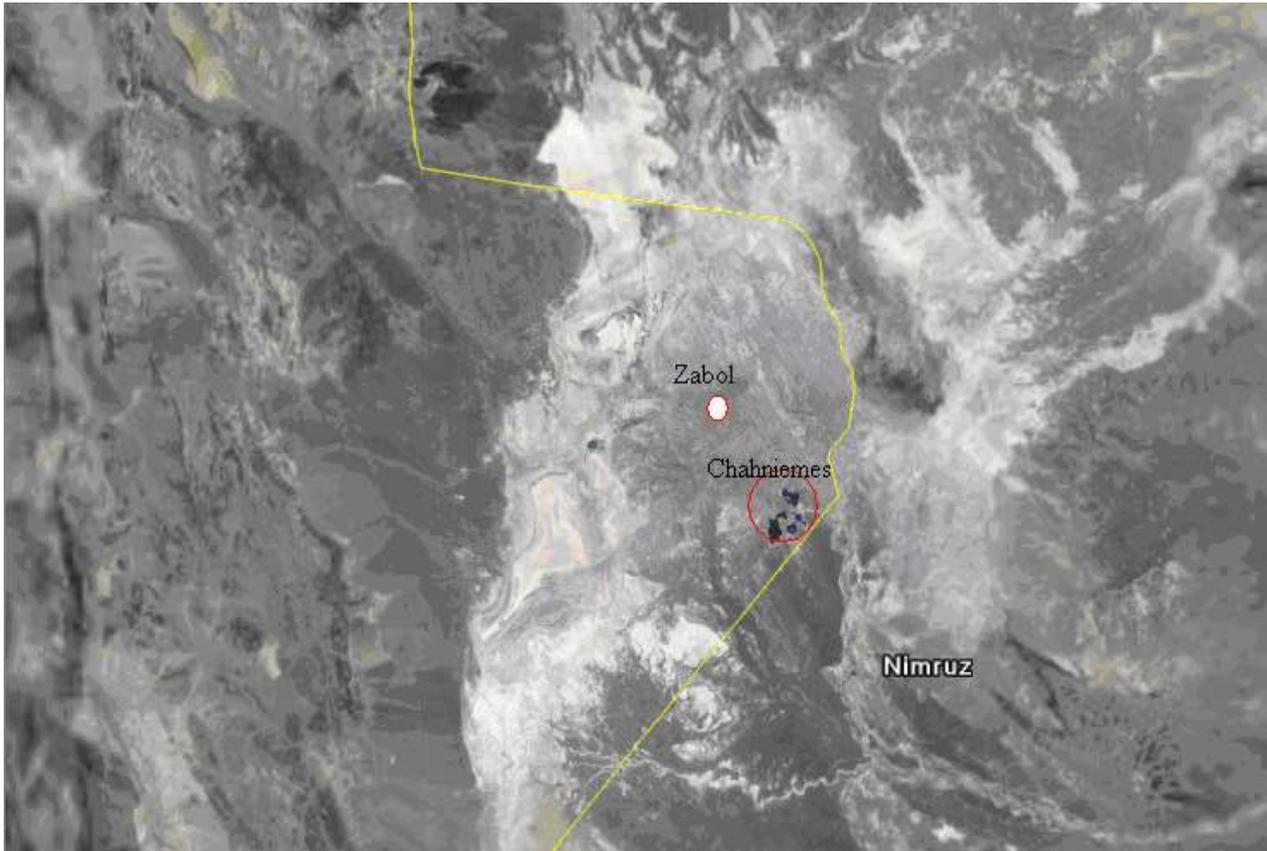
**Fig. 2 – Satellite processed image of the Sistan plain. The Chahnimehs I, 2, 3 and 4 appear as small black patches to the SW of Zabol City. Several NW trending lineaments can be revealed. The alluvial fans to the west of Hamuns Saberi and Helmand are indications that there has been some influx in the west side, too.**
